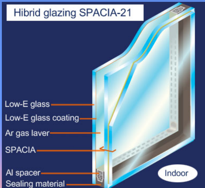
Type 8. Hybrid glazing Low-energy + vacuum glazing
